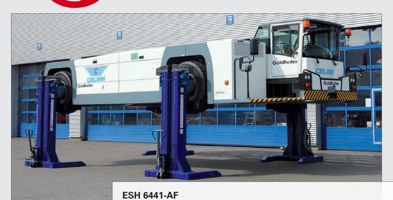
The mobile column lift ESH 6441-AF is designed to lift up all different sizes of tyres
